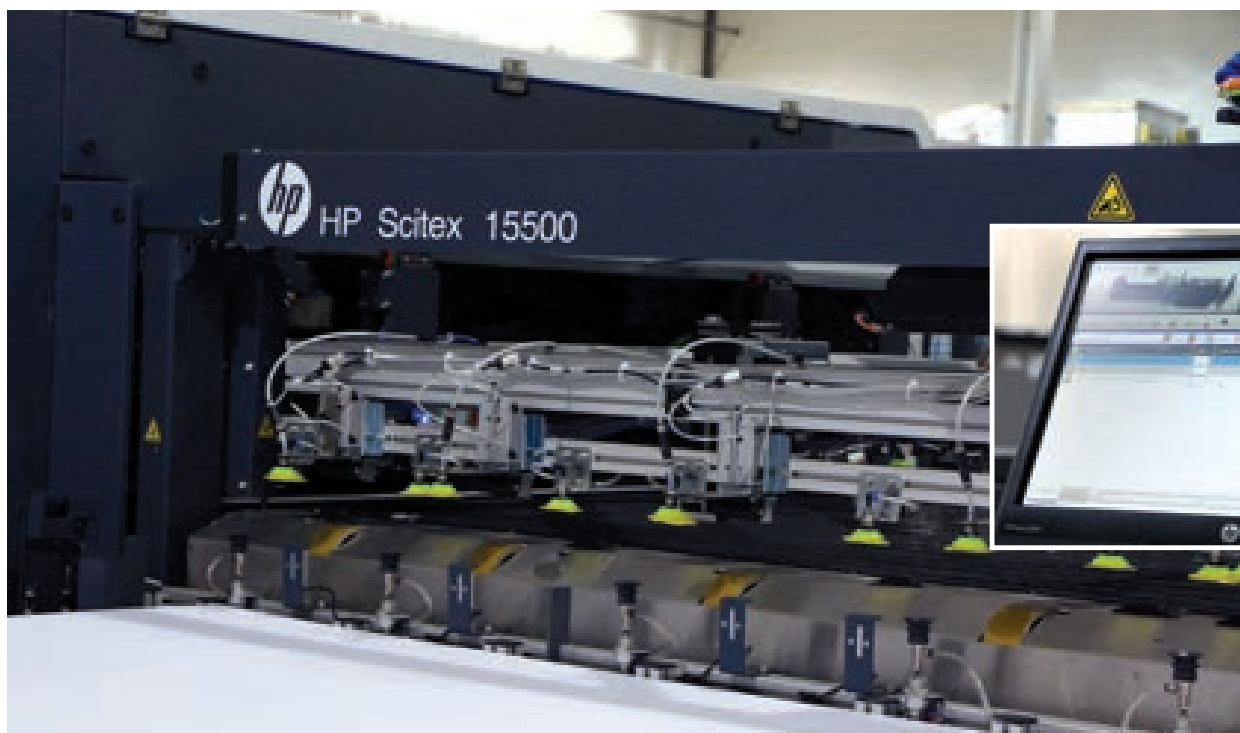
Controlled via an operator-friendly touchscreen interface ( inset ), the HP Scitex 15500 corrugated press uses low-odor HP HDR230 Scitex inks to enable cost-efficient, noncontact printing on paperboards of various grades and thicknesses to provide an optimal solution for short-run production of corrugated trays and other packaging products and displays.
