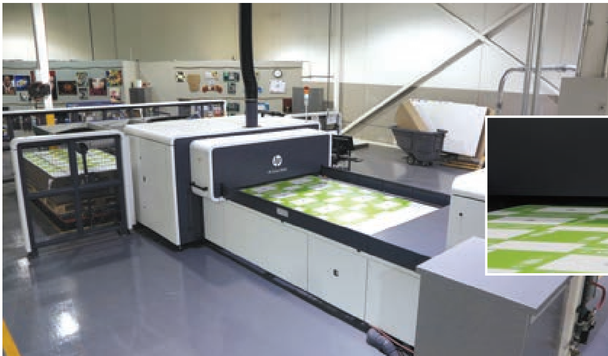
A recent arrival to the Atlantic Packaging Retail Packaging & Display Division's production facility in Toronto's east end, the state-of-the-art HP Scitex 15500 digital printing press is processing a sheet of corrugated board used to make a new batch of carrying trays that will be used by Collective Arts to ship its canned beers to the retail customers.
