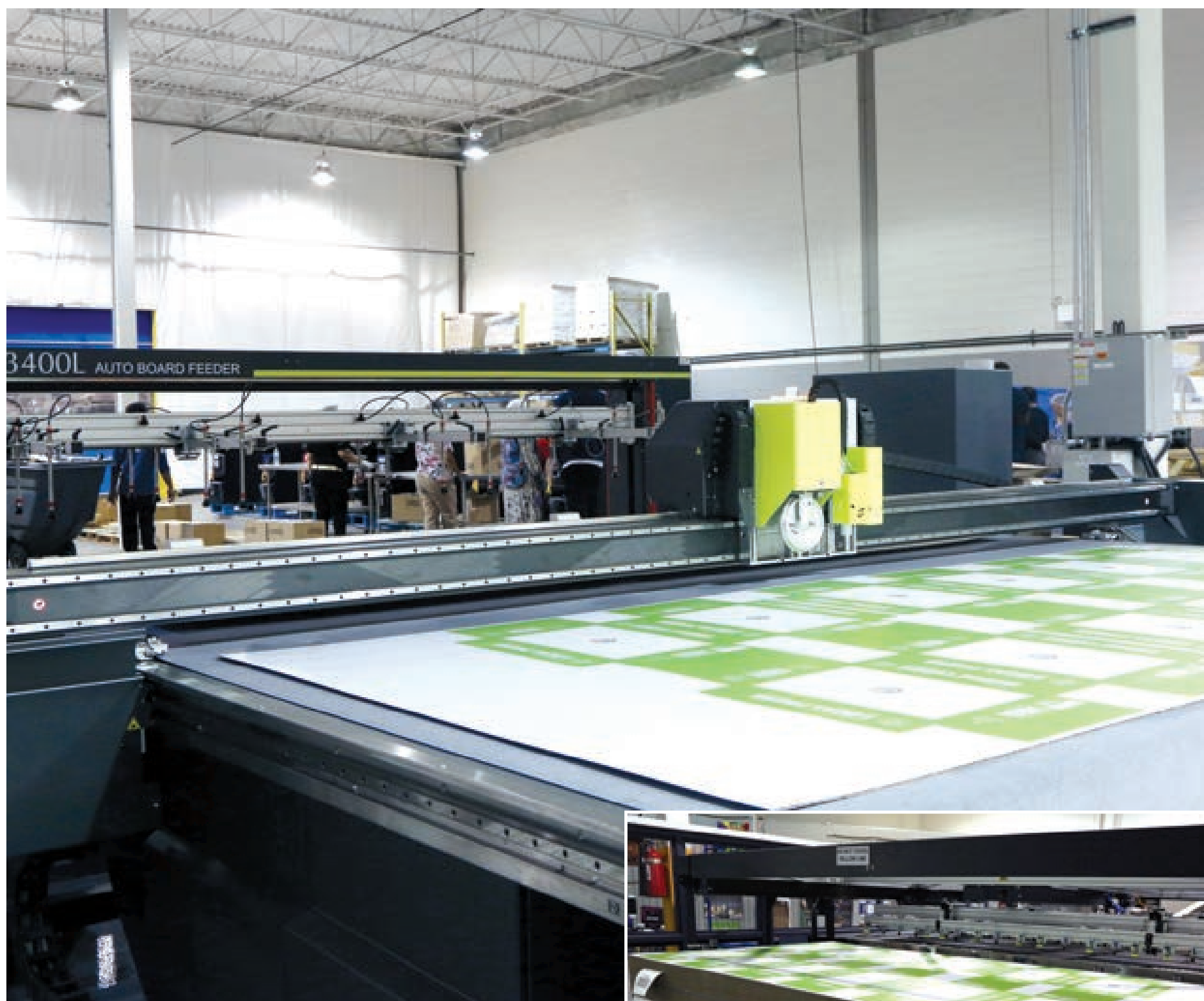
Above: Strategically positioned about 20 feet across from the nearby HP Scitex 15500 corrugated press, the fully-automatic Kongsberg digital flat-bed cutting table is used by the Retail Packaging & Display Division facility to die-cut the digitally-printed sheets.
